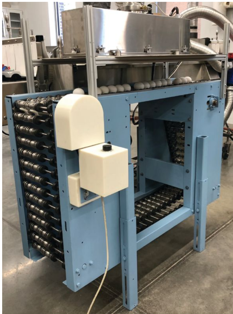
This novel conveyor devised for the experiment was instrumental in achieving acceptable decontamination. As the eggs rotate on their long axis along the way, the entire surface of the eggshell is exposed to the pulsed ultraviolet light energy.
