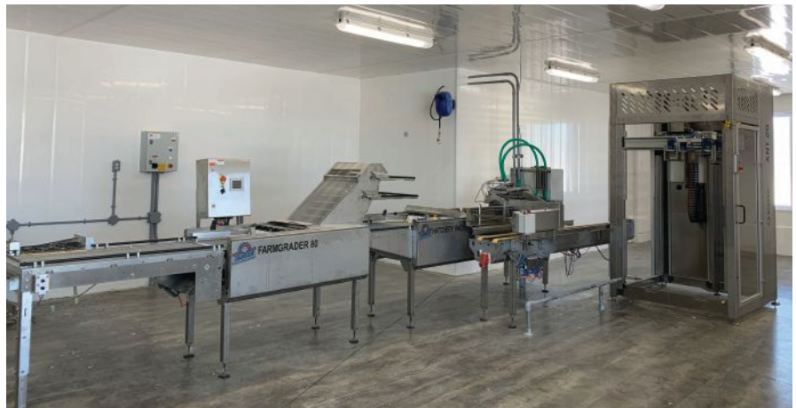
With a Jansen packer and a Kletec trolley loader, their packing process is fully automated.
